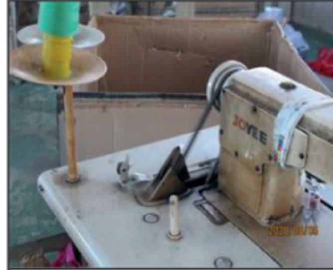
External photo(s) of the production unit(s) 7.17 No belt guard.JPG
